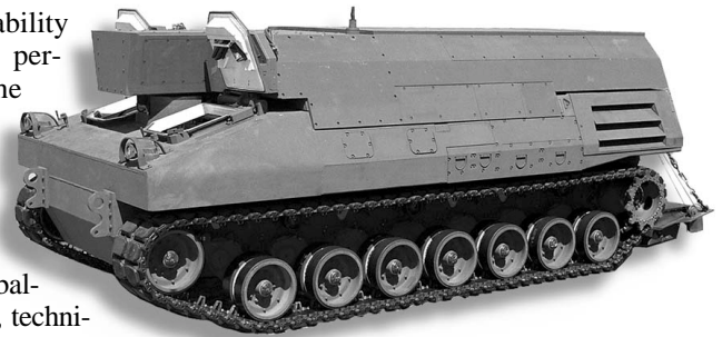
Above: Propellant magazines, part of the automated ammunition handling and loading system of the Crusader howitzer. Below: The resupply vehicle (minus ammunition handling equipment) is the first of the Crusader system prototypes and will be used for mobility testing. It "rolled out" 27 July. (Photo Courtesy of United Defense)
